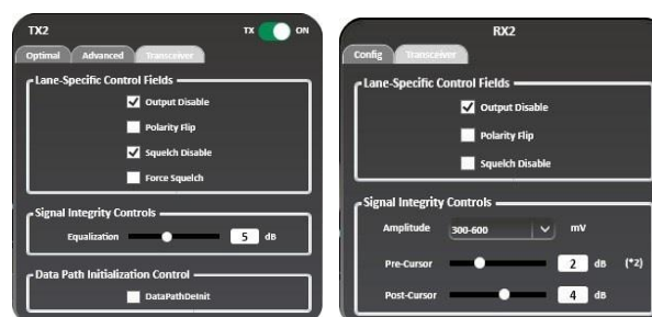
Figure 61: TX-side and RX-side configuration tabs
