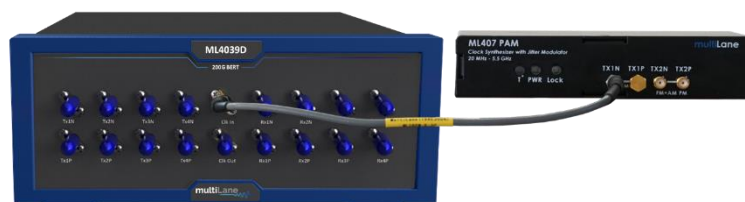
Figure 33: Jitter tolerance hardware setup
